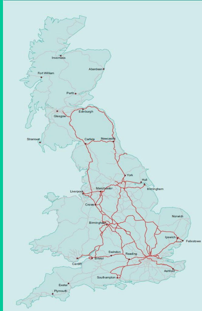
Figure 6.3: W12 gauge clearance aspiration
